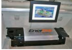
EnerDel has re-powered a Prius with a lithium ion pack
